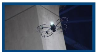
The manufacturer of the drone shown with LED lighting at the Blatnik Bridge in Duluth, MN, advertises its ability to switch between capturing video and still and thermal imagery during the same flight, without landing to change cameras. Source: MnDOT
