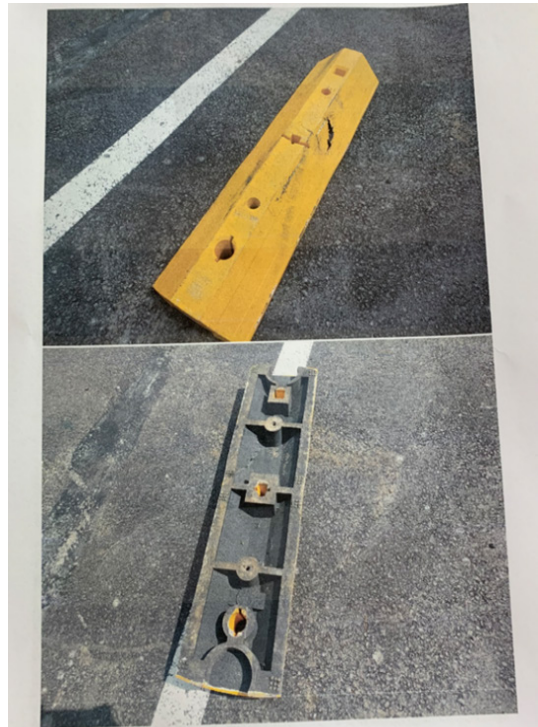
Figure 5: Example of a plastic raised divider that failed in Poland (Source: FHWA)
