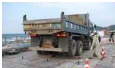
Figure 27. Vibration test using the vehicle falling method.
