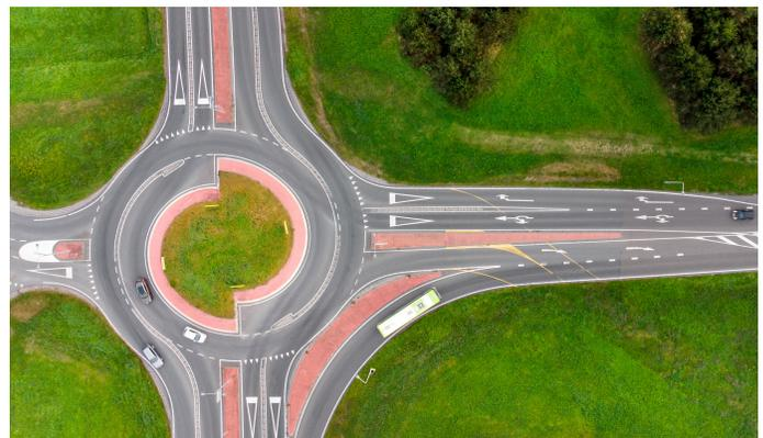
**FIGURE 1.** AERIAL VIEW OF A TURBO ROUNDABOUT IN THE NETHERLANDS. **SOURCE:** USDOT/GETTY
