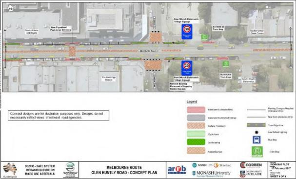
Figure 4. Proposed concept design for a section of Glen Huntly Road (Source: <u>Austroads</u>)
