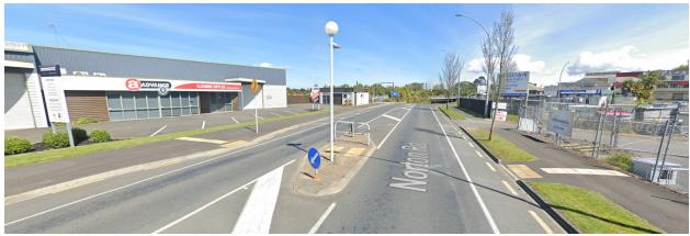
Figure 6: Norton Road with protected median refuge including a raised island, signs, overhead lighting, curb cuts, and tactile dome warning strips (Source: <u>Google Maps</u>)
