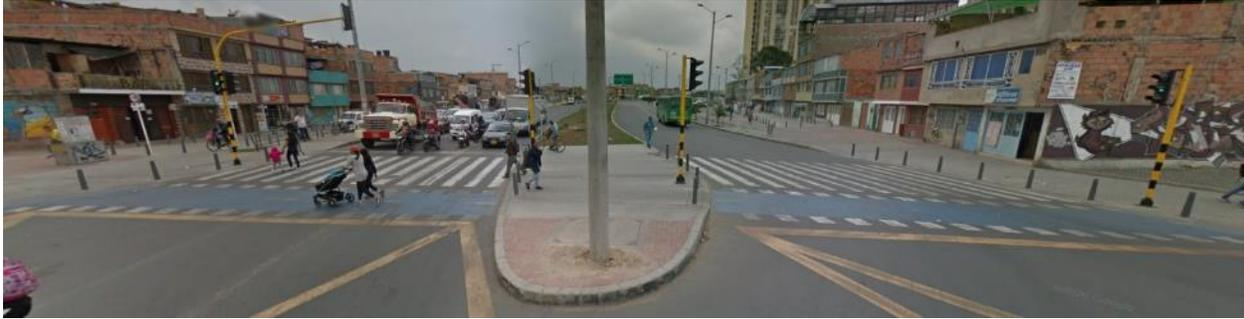
Figure 21: Typical post-project crossing configuration - painted crosswalks and bike-walks, bollards, and brightly painted signal poles (Source: [Google Maps](#))
