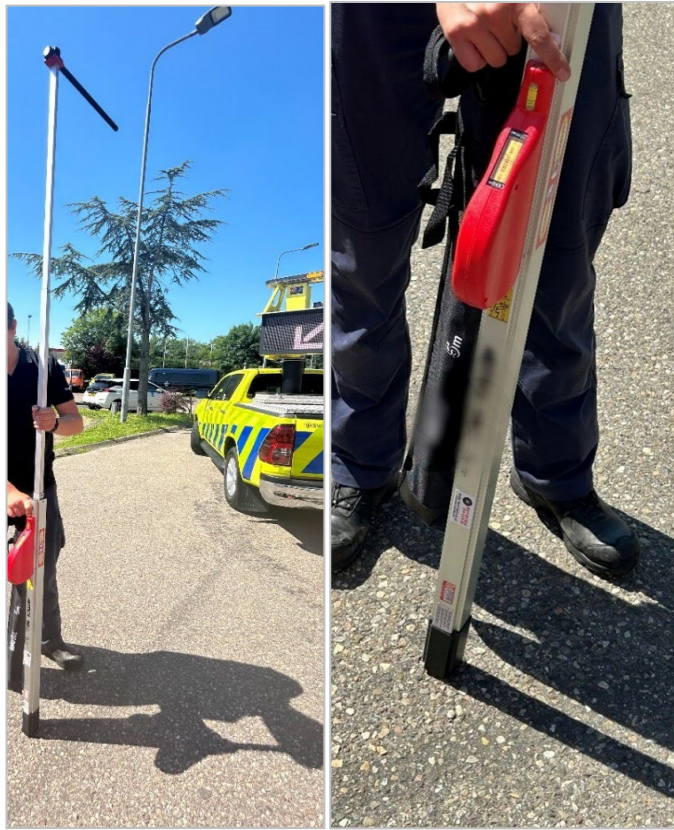
Figure 22: Rijkswaterstaat Vehicle Height Measuring Device
