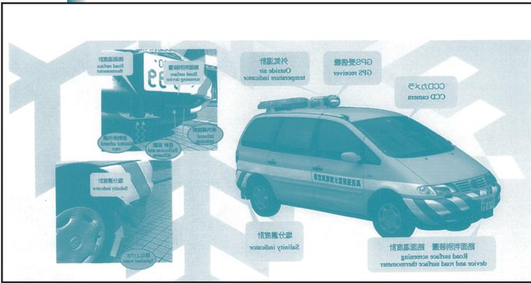
Figure 2. The Japan Highway Public Corporation uses specially equipped patrol vehicles to monitor wintertime road surface conditions.
