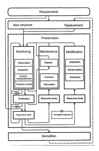
*Figure 5 Flow chart for preservation of engineering structures in water (7).*
