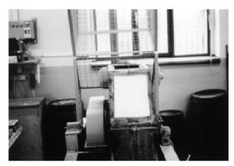
Figure 12. Abrasion test apparatus—BAW, Karlsruhe, Germany.
