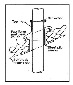
Figure 20. Flexible collar arrangement at a pile to seal the joint with a mattress.
