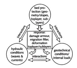
*Figure 1.* Soil-water-structure interaction (SOWAS concept) (8, 22).
