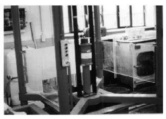
Figure 11. Impact test apparatus—BAW, Karlsruhe, Germany.
