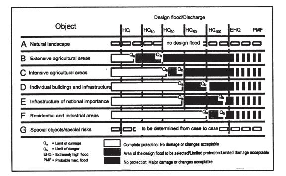
*Figure 2.* Differential safety concept—according to safety objectives a variable design flood can be applied for flood control works (23).
