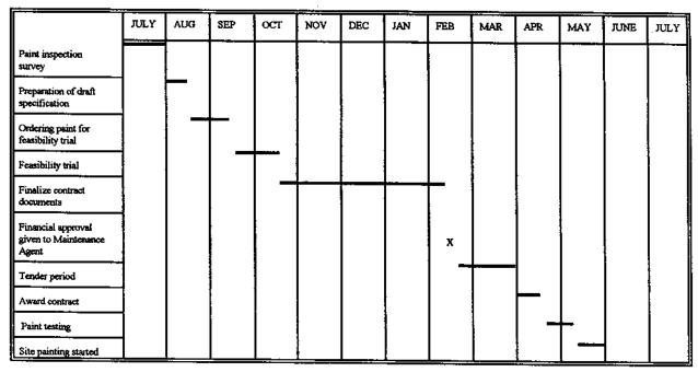
Note: Guide based on the assumption that the paint inspection survey and feasibility trial are carried out in the same year and the maintenance painting contract started the following year.
