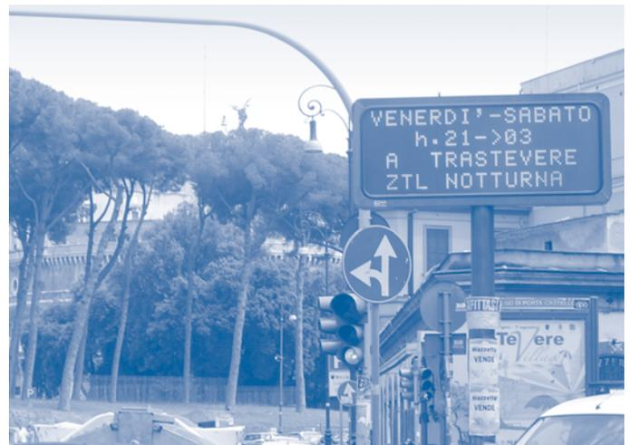
Figure 14. Variable message sign at ZTL access point.
