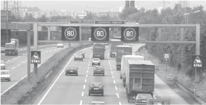
Figure 14. Congestion warning system in Germany. (23)
