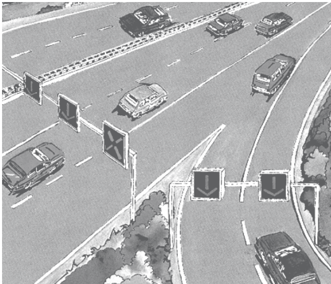
Figure 18. Junction control schematic in Germany. (21)
