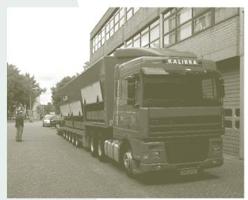
Figure 14. The Netherlands: dynamic calibration vehicle.
