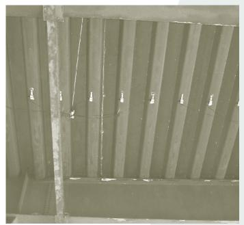
Figure 18. France: bridge WIM system test site.
