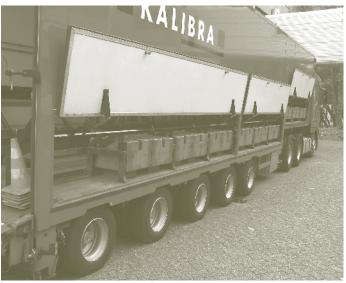
Figure 15. The Netherlands: dynamic calibration vehicle.
