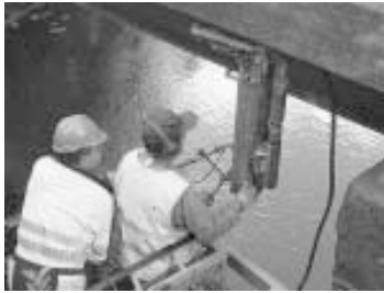
Figure 2. A core sample is being taken of one of the reference bridges near Kemi in Northern Finland.
