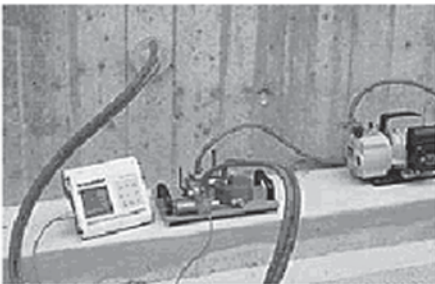
Figure 48. Torrent permeability meter. (Proceq USA 2004)
