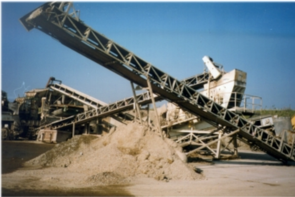
Figure 10. The C&D crushing process at the RGS 90 A/S materials processing plant in Denmark.
