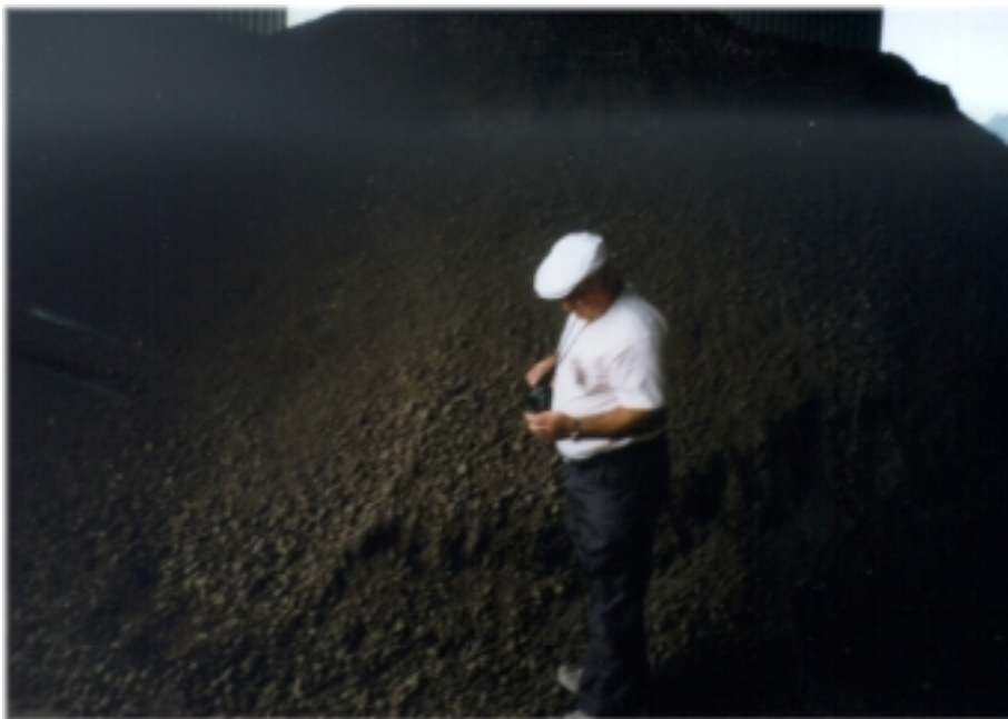
Figure 14. RAP containing tar at the DEUTAG asphalt plant in Germany. The plant is experimenting with processing and use of different recycled materials. The RAP containing tar will be tested in a foamed bitumen application.
