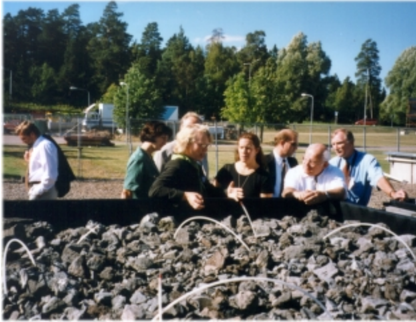
Figure 8. Lysimeters used at SGI for field leaching of candidate recycled materials.
