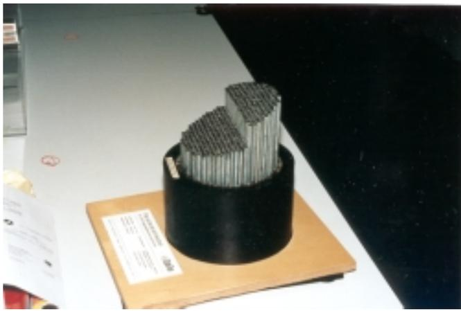
Figure 33. Cable stay of Sunniberg Bridge, Switzerland, consists of parallel wires in a matrix inside a thick-walled PE pipe.
